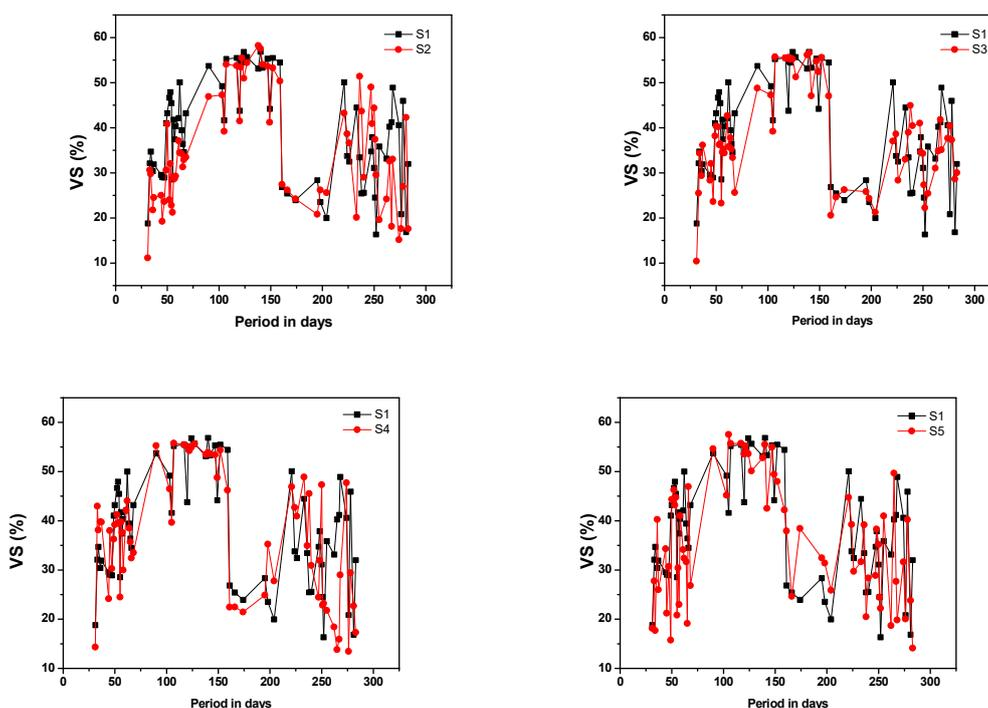
Fig.5 Volatile solids variation during sludge feeding period in Pilot-scales STW system
