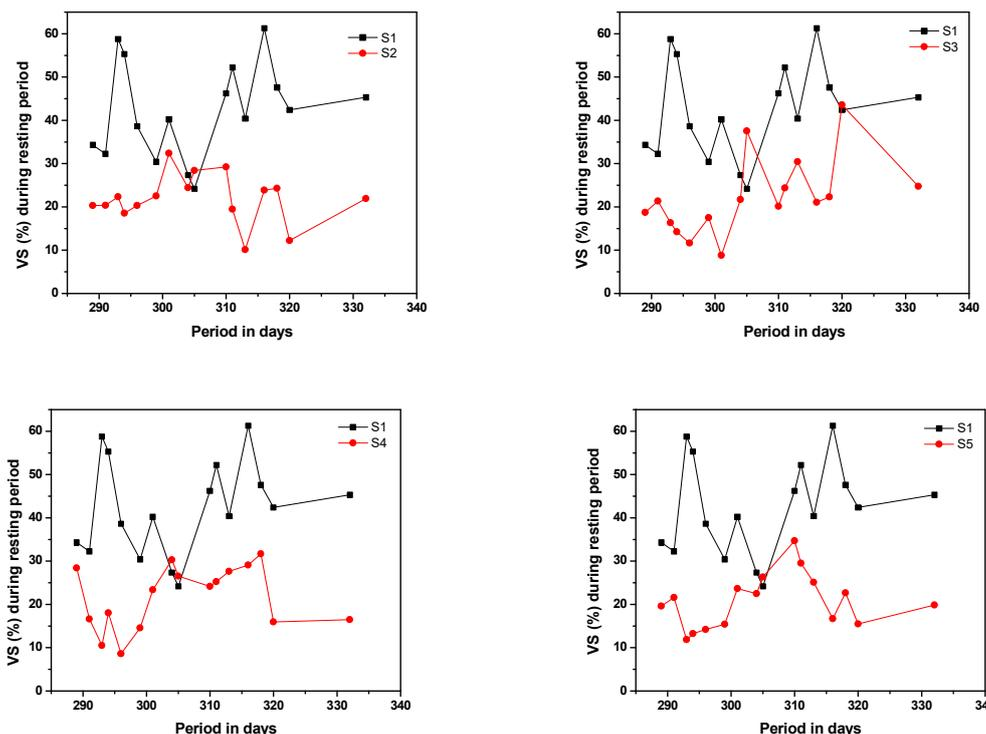
Fig.6 Volatile solids variation during final resting period in Pilot-scales STW system
