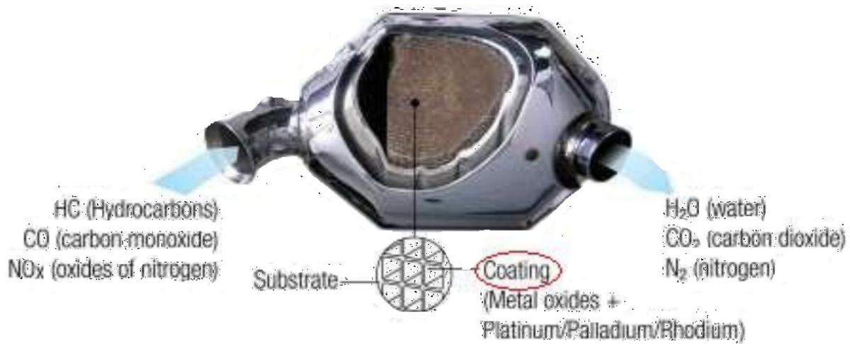
**Figure 2.2 :** Gases in Catalytic Converter
