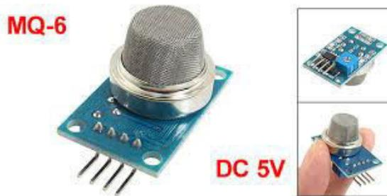
Fig4: MQ 6 Sensor
