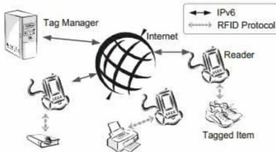
Figure 4 Connecting RFID Tags to IoT
